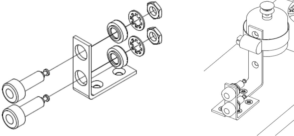
13. Attach this power input assembly to the plywood base just as you did the motor mount: mark the hole locations, pre-drill with a 1/16" bit, and use two #6 x 0.75" wood screws. Where you put this is not critical. It just has to be close enough to the motor that the wires reach.
