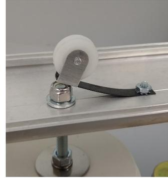
The mounting hole should be large enough to accept a #8 screw, which—officially—should be done with a #16 drill. But you most likely don't have a set of number drills, so use a 3/32" drill instead.
