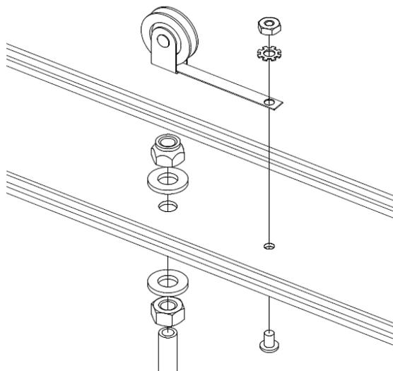
12. Use a 3/8" drill to enlarge two adjacent holes in the 1.5" corner brace. This will go better if the brace is clamped in a vise. Unfortunately these holes are not quite 3/4" apart. If you don't know why that is unfortunate, then never mind. It will make no difference to you. Then assemble the two banana plug receptacles onto the brace as shown. I used one red receptacle and one black receptacle because I am that way, but the electrons don't really care about the color.
